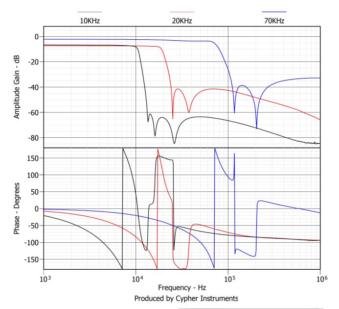
Three low pass filter modules were tested using the C60. These filters have an Elliptic response, which means that they have stop band transmission zeros. The phase response performs a rapid 180° transition when the test frequency passes through a 'perfect' zero.
