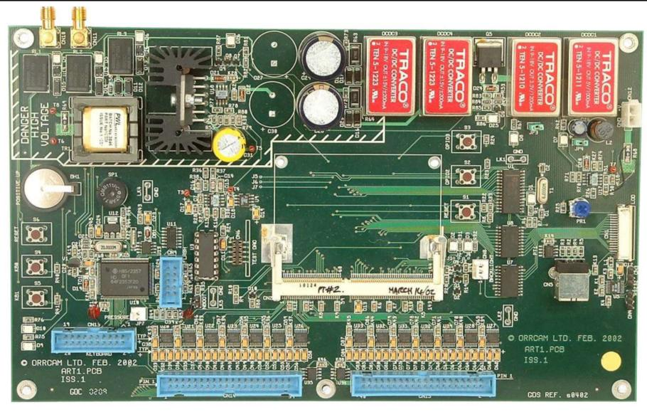
The picture above shows the mother board of a 28 channel NDT product. The board captured 28 channels of ultrasonic signals, which it stored on a 'micro engine'. The board also has a display and keyboard, a clock calendar, temperature sensor, GPS receiver, battery voltage and current monitor, a power supply switcher, a flash micro controller, USB A & B ports, serial I/O and a waveform generator with 400Vpp @ 1 Amp power amplifier.
