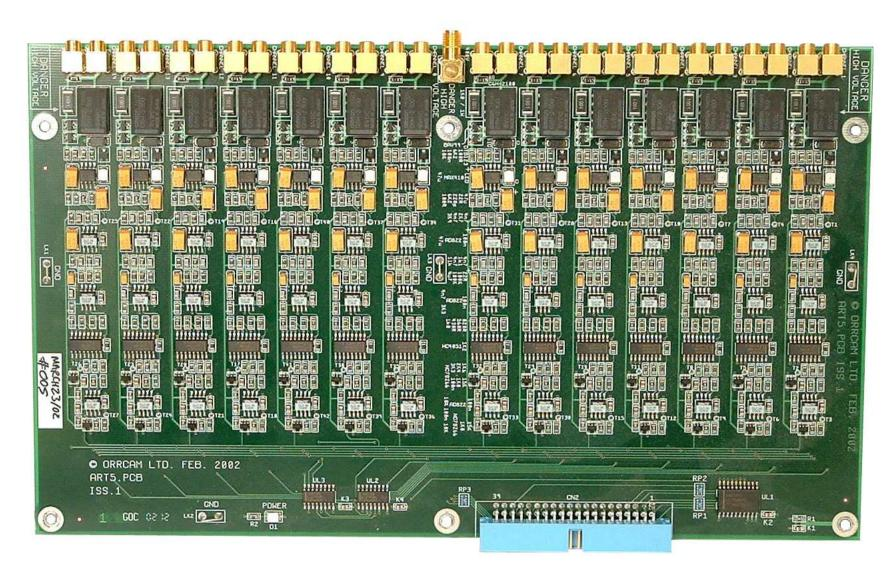
The picture above shows a 14 input channel NDT analogue board. Each channel performed a pulse/echo function, with a 400Vpp output voltage withstanding capability, a voltage protected low noise amplifier stage, a digitally controlled logarithmic gain stage and switched active filtering. The NDT system had two of these boards to perform 28 channels of analysis.
