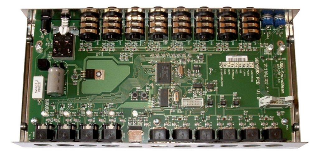
The picture above shows a prototype of a music product. The electronics consists of a flash microcontroller, a USB interface chip and not much else, apart from 21 connectors! The unit measures distance with an ultrasonic ranging mechanism and converts this information into control data for musical sound generators.
