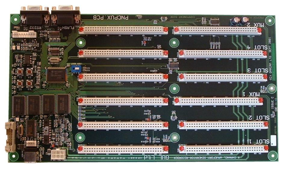
The picture above shows a 4 channel NDT product. The electronics on this mother board was designed to be minimal. It has a flash microcontroller, RAM, USB interface, two RS232 interfaces and a DC control DAC. The system was battery powered and so low power was important. Multiplexer and I/O boards plug into the connectors.
