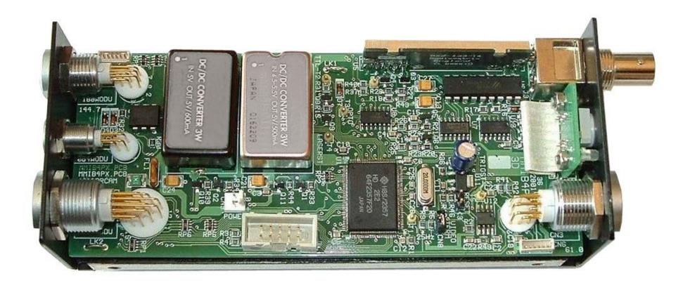
The product shown above is an industrial control unit. It incorporates a power management system, a radio remote control receiver, a video interface and all the connectors to the rest of the system. A flash micro controller handles all communications to the PC and from the acquisition hardware.
