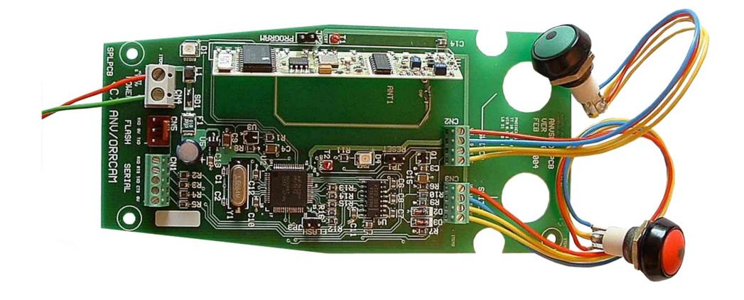
The product shown above is a remote control interface to a sound pressure level meter. The board uses a small flash microcontroller to generate RS232 communications between the meter and the panel switches and the RF remote control.
